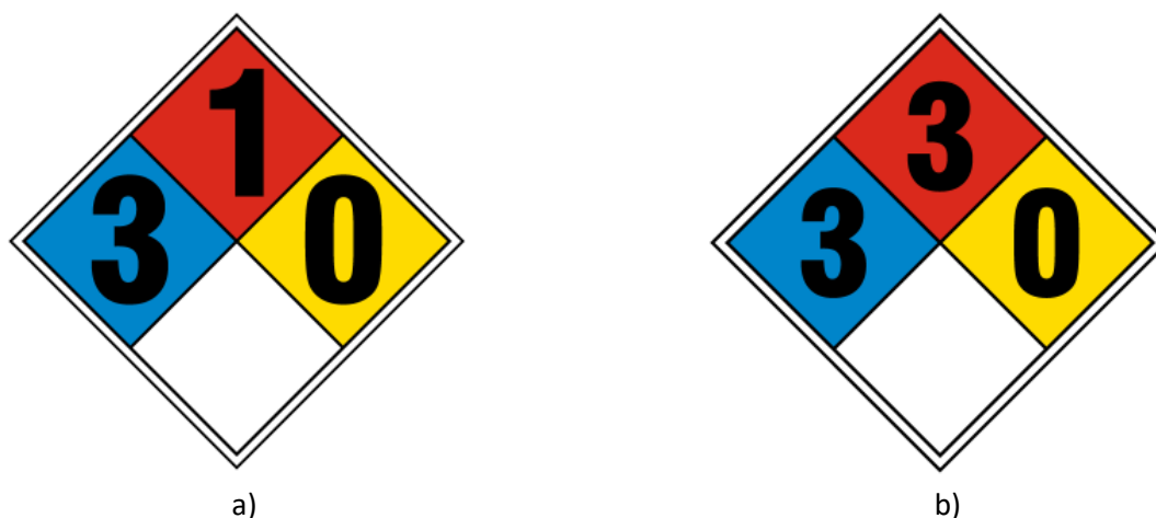
Figure 1. NFPA 704 hazard diamond for anhydrous ammonia showing fire (red), health (blue), instability (yellow), and specific (white) hazards for (a) open and (b) confined locations [8]
