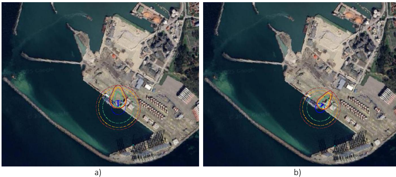
Figure 25. a) Toxic outdoor probit footprint for scenario 2.1 b) Toxic outdoor probit footprint for scenario 2.3
