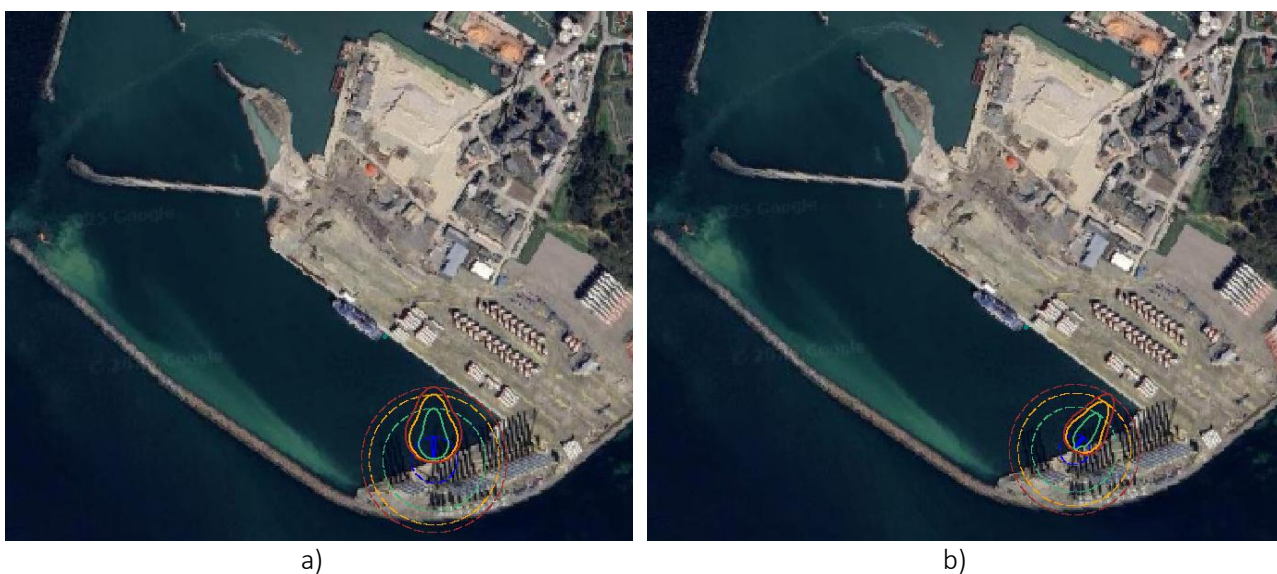
Figure 26. a) Toxic outdoor probit footprint for scenario 3.1 b) Toxic outdoor probit footprint for scenario 3.3
